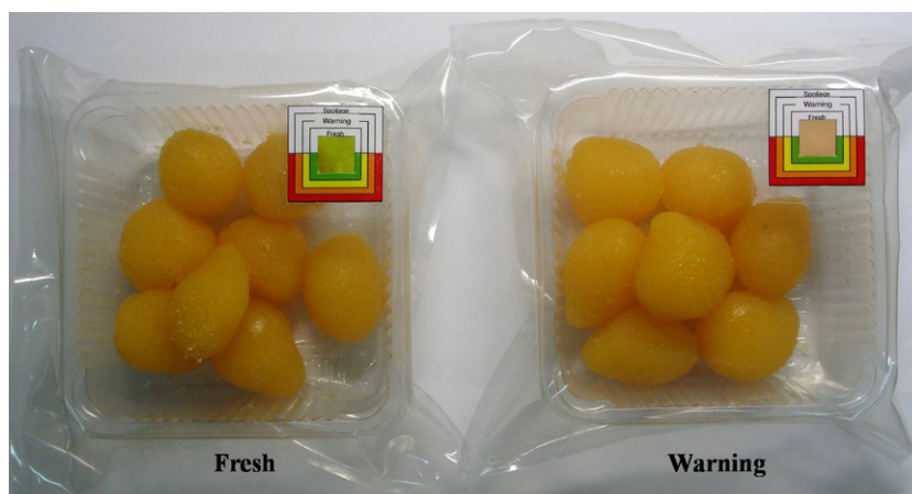
Fig. 6. Packaged golden drop with food spoilage indicator label. Green = fresh; orange = warning. (For interpretation of the references to color in this figure legend, the reader is referred to the web version of the article.)
